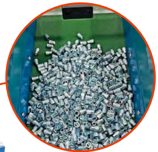
Storage magazine (5,000 rivets capacity)
