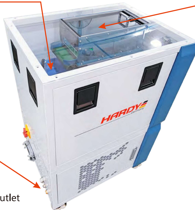
Storage magazine (5,000 rivets capacity)
